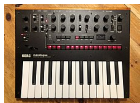
The Korg Monologue is a monophonic synthesizer with two VCOs.
