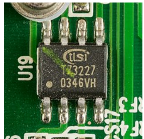
27 MHz VCXO clock generator IC (TLSI T73227), used in a DVB-T set-top box.
